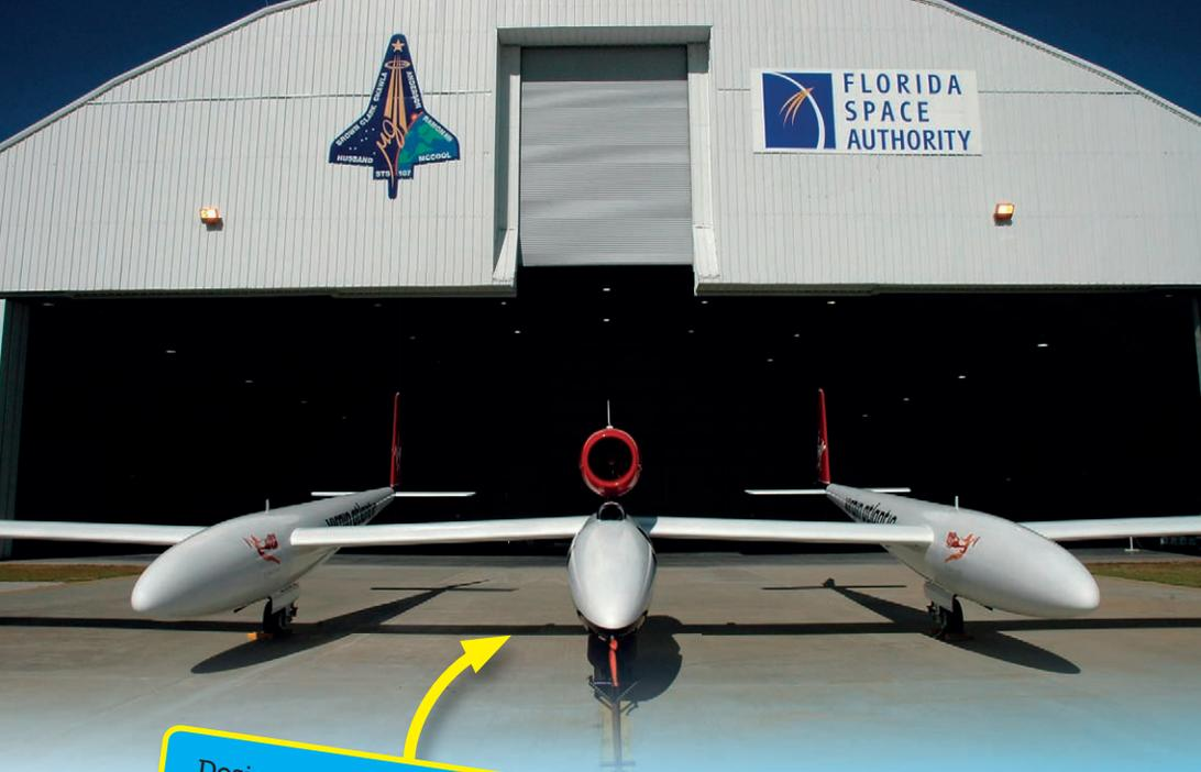
Designed and built for Fossett in the United States, GlobalFlyer was made of plastic and carbon fiber, with a single turbojet engine.
